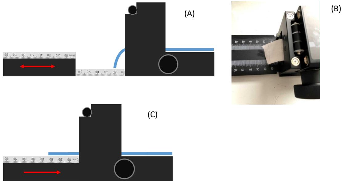
The CLO KIT does not distinguish between face up and down and fabrics can be tested randomly. This is in contrast with the standard procedures, such as BS 3356:1990 [22] and ASTM D1388-96 (2002) [30], where both sides are tested. As well as to the significant differences between the face and back drape coefficient (DC) that some fabrics have, the DC is closely related to the bending length [19].
