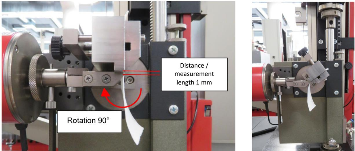
**FIGURE 20: BENDING STRAIN-STRESS BEHAVIOR**
