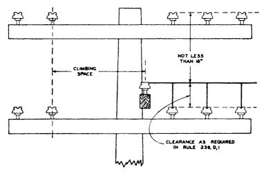
Fig 9 Obstruction of working space by buckarm.
