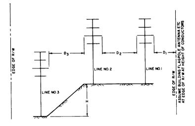
Fig IR 158 To determine  $D_1$ ,  $D_2$ , and  $D_3$  as required by the NESC.
