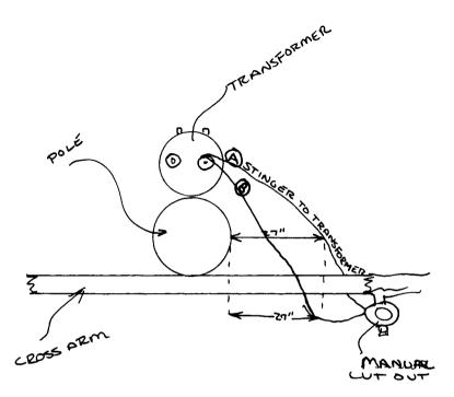
Fig IR 176-3. (1) Does climbing space extend into this stinger wire if mounted in the position of stinger A? (2) Does climbing space extend into this stinger wire if mounted in the position of stinger B?
