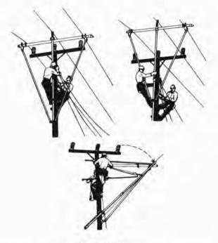
Fig IR 167-5 Maintenance by "jacking" conductors up or toward the side.
