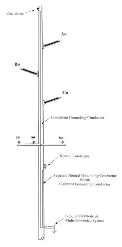
Figure 1—Typical wood transmission structure with distribution underbuild
