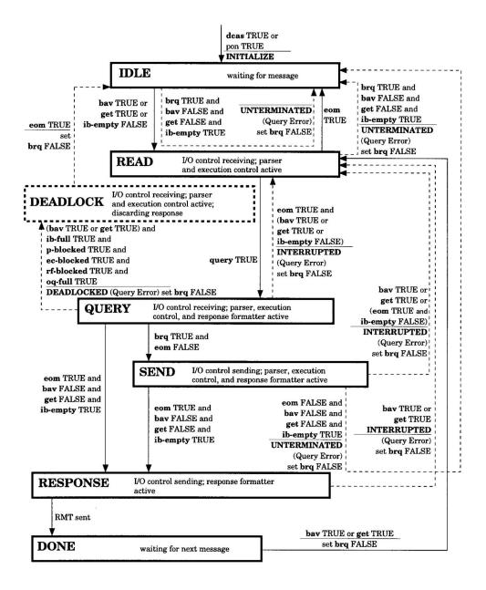
Figure 6-4—Message Exchange Control State Diagram (Complete)
