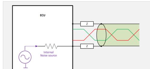
← Resistive coupling: independent of coupling frequency
