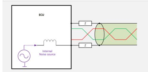
← Inductive coupling: coupling  $\propto$  1/frequency
