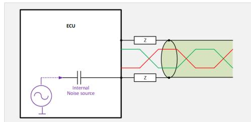
← Capacitive coupling: coupling  $\propto$  frequency
