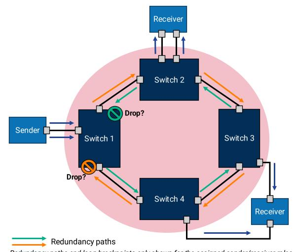
Redundancy paths and loop breakpoints only shown for the assigned sender/receiver roles.
