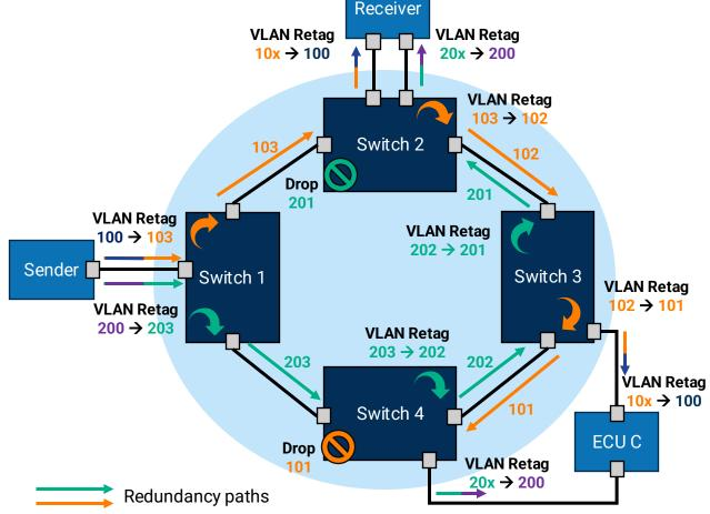
Redundancy paths and loop breakpoints only shown for the assigned sender/receiver roles. VLAN retagging performed always on switch egress as specified in OA TC11.
