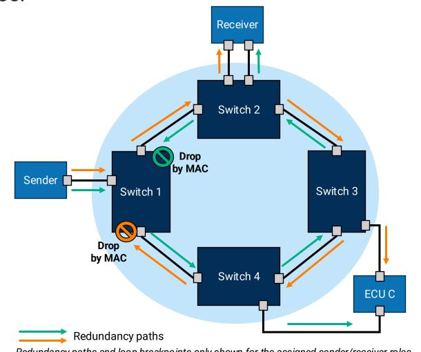
Redundancy paths and loop breakpoints only shown for the assigned sender/receiver roles.
