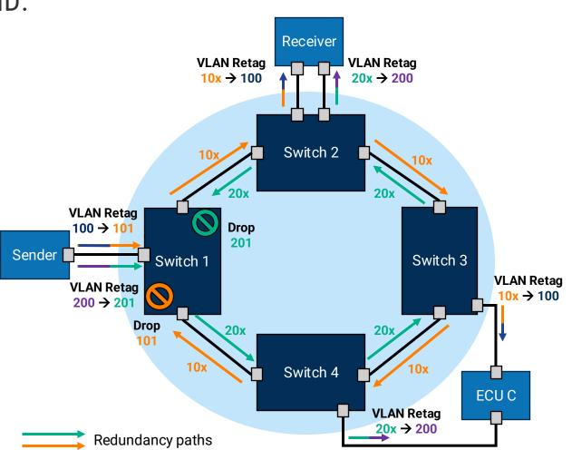
Redundancy paths and loop breakpoints only shown for the assigned sender/receiver roles. VLAN retagging performed always on switch egress as specified in OA TC11.
