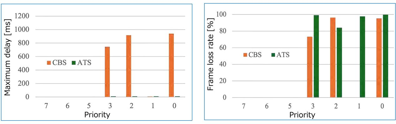
Since frames are no longer held in the token bucket due to bursts, the maximum delay can be suppressed entirely in ATS. While ATS suppresses the maximum delay, frame loss occurs in ATS even though there was no frame loss in CBS.
