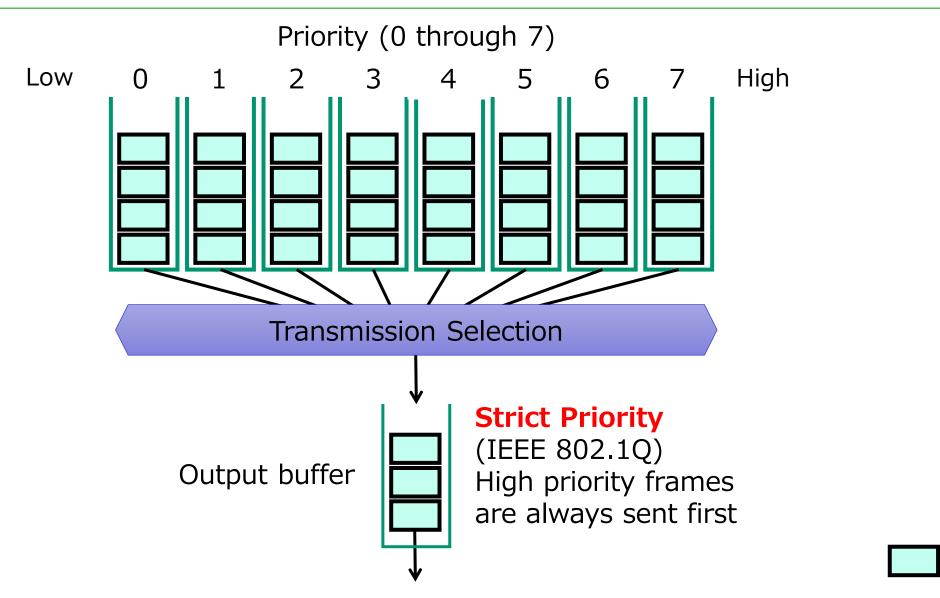
Prioritizing only high-priority data can result in bursts of traffic that can cause flooding in a zone.
