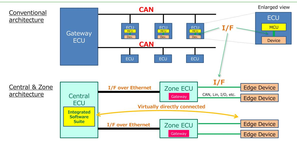
The C&Z architecture will significantly change the data transmission through channels.
