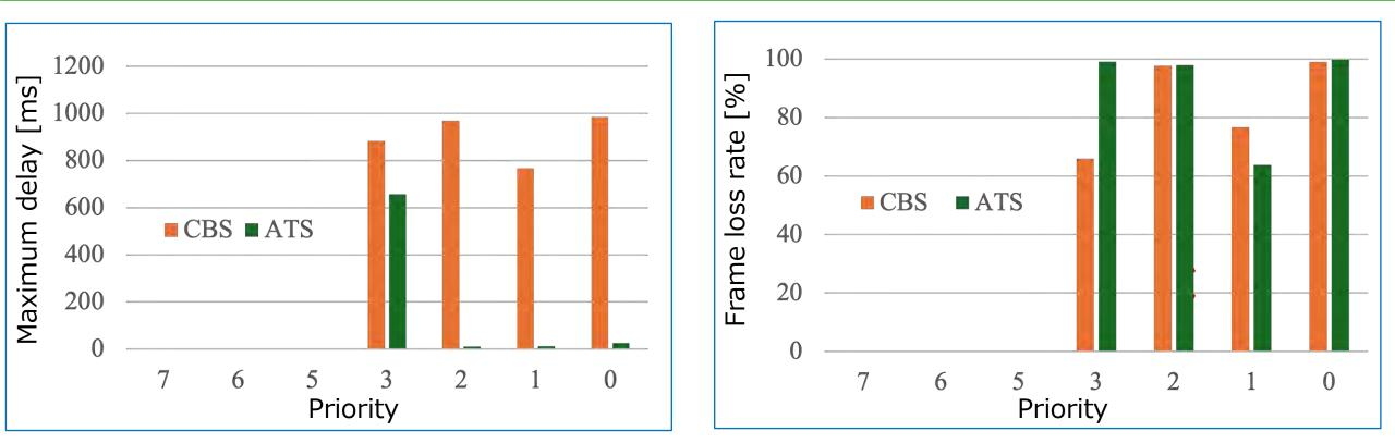
By setting Committed Burst Size, ATS can suppress the maximum delay more than CBS. Additionally, the maximum delay can be managed by adjusting the Committed Burst Size.
